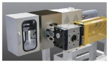
Double layer auto filter change, Italian gear pump design for quantitative material supply.
