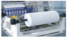
Unwinding unit configures with missing fabric detection and automatic unwinding change device; not only running with magnetic brakes, pneumatic disc brakes can be used as optional.
