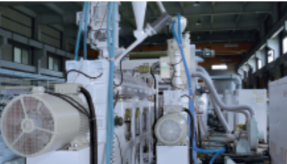
The double extrusion goes through the feed block device and the special T-die runner to make the three-layer A.B.A co-extrusion.
