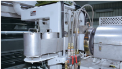
Double-layer automatic network switching device, can choose plastic pressure control network change and timing control network change.
