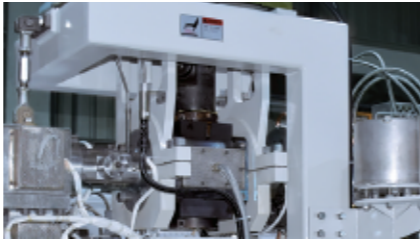
Melt pump (optional), its function is to maintain the quality and stability of the extrusion.
