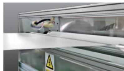
Use device of electrostatic electret technology, and the static electricity is absorbed in the meltblown nonwoven fiber to improve filtering performance.
