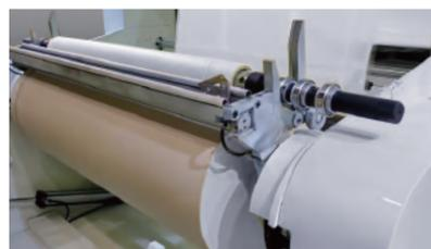
The winder is designed for automatic length calculation, cloth cutting and roll change, which is easy to operate.
