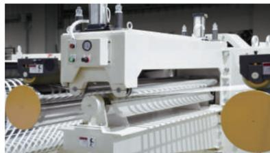
Fibrillating device with pneumatic lifting.
