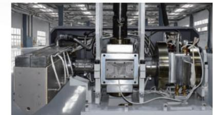
Double layer auto-screen changer, metering gear pump and T-die thermal insulation design.
