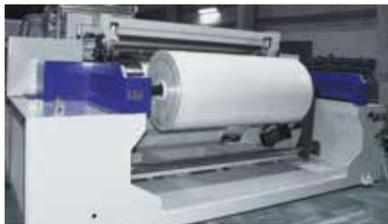
The winding unit is equipped with automatic length measuring and cutting function for fabric roll change.
