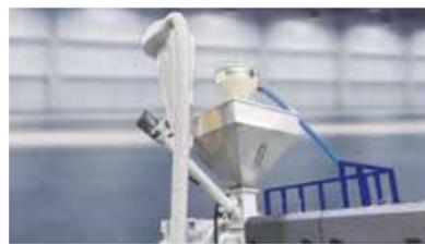
Edge material recycling device, where the trimmed material is crushed and directly mixed with the raw material before extrusion.
