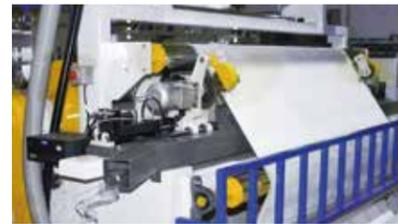
Automatic EPC edge trimming and cutting device, with provision to reserve extra film width without cutting into the fabric.
