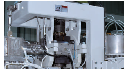
Melt pump (optional), its function is to maintain the quality and stability of the extrusion.
