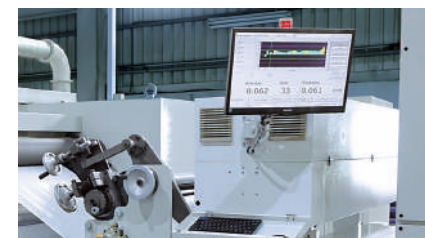
MEC-P-150 Thickness measuring machine, the use of Germany imported infrared MF electric eye, measurement accuracy of \pm 5\mu\text{m} , no radiation problems.
