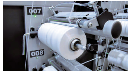
Inverter type and automatic tension control winder, the light-weight design of the tape guide slide achieves power saving performance, and the winding shaft is equipped with a hooking device to facilitate the roll change.
