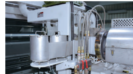
Double-layer automatic network switching device, can choose plastic pressure control network change and timing control network change.
