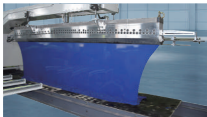
The wide-width T-Die head undergoes precise runner design and machining to ensure uniform film flow.
