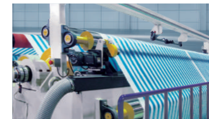
Trimming and center slitting device.
