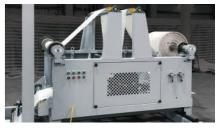
The unwinder is equipped with cloth roll missing cloth detection and automatic roll change design, make operations more convenient.
