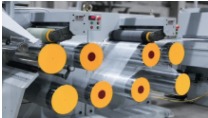
The process design of stretching and preheating roller make high denier tape to achieve the tape stability.
