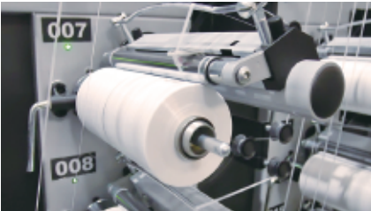
Inverter type and automatic tension control winder, the light-weight design of the tape guide slide achieves power saving performance, and the winding shaft is equipped with a hooking device to facilitate the roll change.
