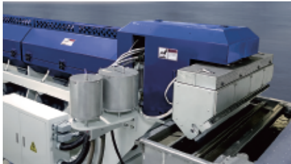
Double layer auto filter change and T-die thermal insulation design.
