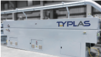
The design of air volume rectifier and uniform heating inside the extended oven makes the high denier tape achieve the effect of extended average.
