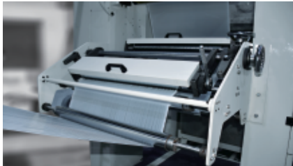
High denier tape adopts two-component knife with non-stop design and swing device to increase production efficiency and also extend blade life.
