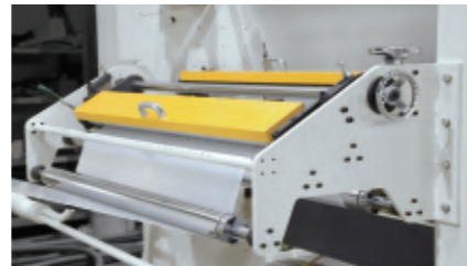
Front and rear two-component strip edge device can be exchange for increased productivity.
