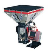
MAGUIRE blender(optional), and its function is to automatically cut and mix according to the proportion of raw materials.
