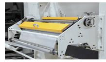
Front and rear two-component strip edge device can be exchange for increased productivity.
