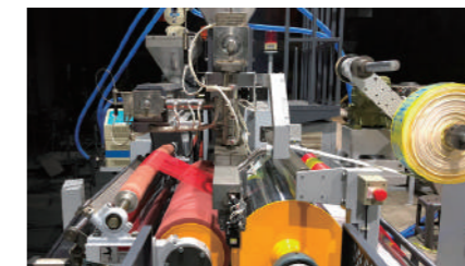
Simple film flow design and dual extrusion achieve high efficiency and energy saving.
