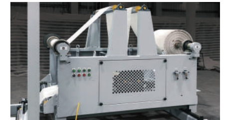
The unwinder is equipped with cloth roll missing cloth detection and automatic roll change design, make operations more convenient.
