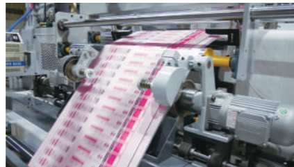
EPC automatic edge cutter device, color film can effectively align and adjust the trim size.
