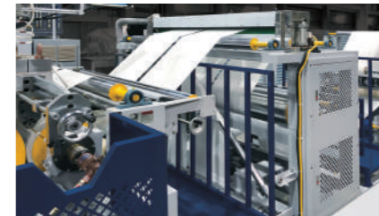
PP Surface treatment corona and PP woven bag turn bar device.
