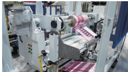
The unwinder of BOPP sandwich laminating machine, and the take up motion of unwinder can range into two types which are speed decrease or not decrease.
