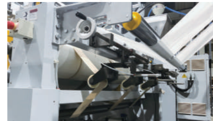
Teflon tape device with belt type, two side or unilateral adjustments.
