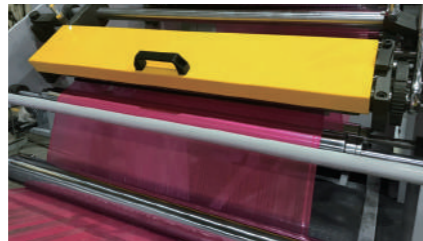
5 sets slitting knife with swing device and non-stop design.
