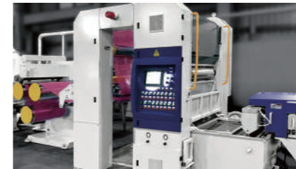
Quench take-up unit, with extrusion device, film cooling forming, and water removal system to keep the film even.
