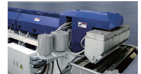
Double layer auto filter change and T-die thermal insulation design.
