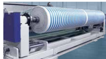
The wide-width unwinding machine adopts a fixed-seat movable design, suitable for various widths of fabric rolls.
