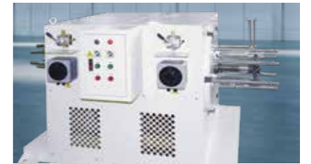
Dual-wheel pneumatic edge-rolling machine facilitates easy removal of waste fabric edges.
